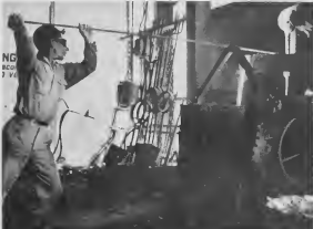
ESTEVAN CROES is "butting the cupola" (that is, stopping the flow of cast iron from the furnace to the ladle) during the last use of the coke-and-air fired furnace.
